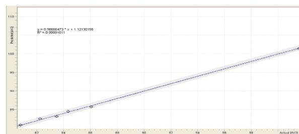
Figure 4. PLS calibration model for correlation between actual and FTIR predicted value of acid value.
